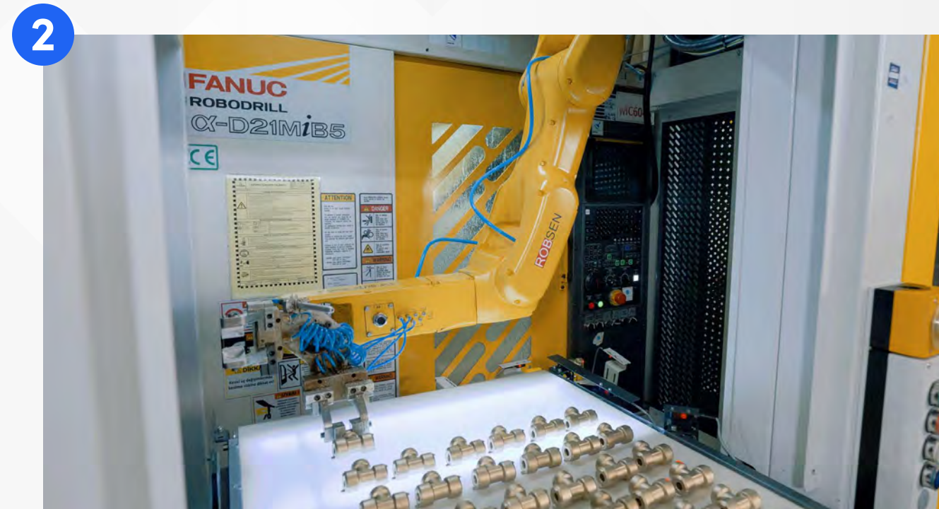
The robot picks reliably from random orientations.
